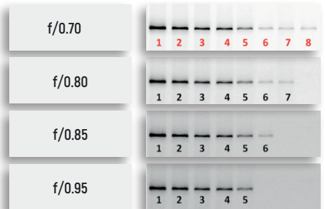
Figure2. The HSR technology provides a better sensitivity by reducing the noise ground level. By keeping the background to its lowest floor level, the very faint signal can easily be detected and quantified.
